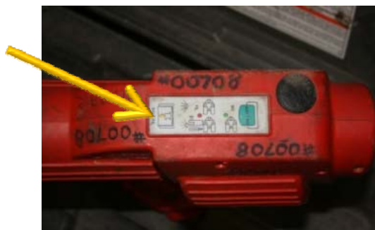
Arrow shows the area where the yellow LED signals the need for recalibration
