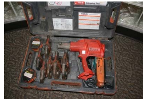
Pro-press; handles 1/2" – 2" copper pipe
